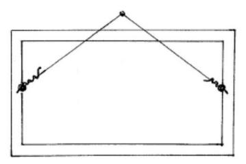
Wire too long, no tape or shrink tubing on wire.
